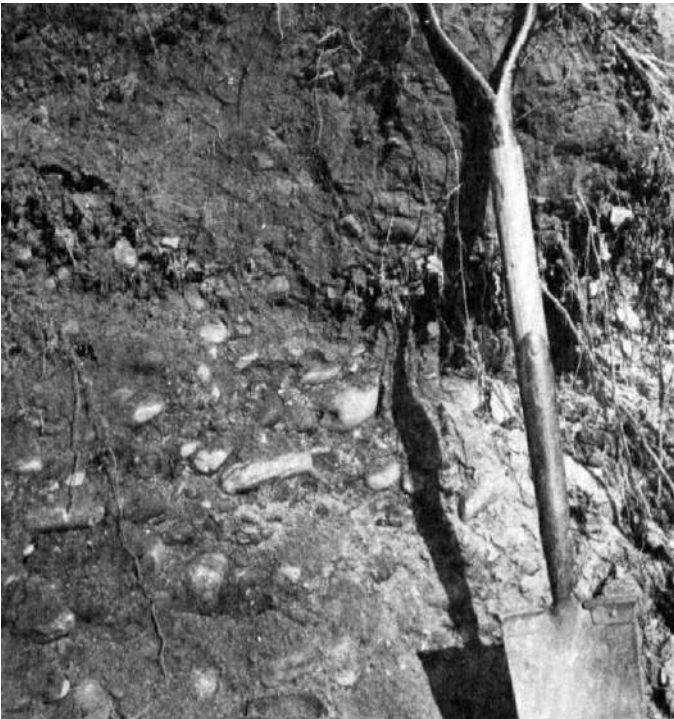
Figure 16.—Profile of Masardis gravelly fine sandy loam, 3 to 8 percent slopes. The rounded coarse fragments are an indication that the soil formed in glaciofluvial deposits.
